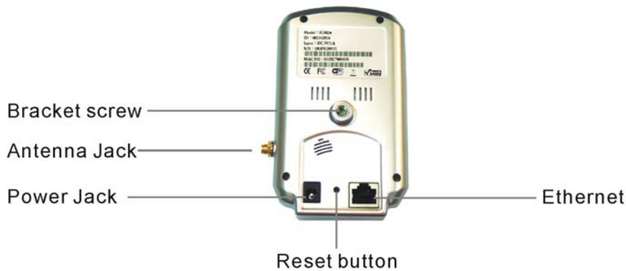
Figure 2-2: Major components in the back panel
